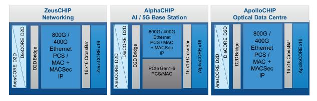
**ZeusCHIP:** Contains the industry leading DieCORE100 or AresCORE D2D interface and can be matched with AthenaCORE200 or ZeusCORE100 to meet the needs of top-of rack networking interconnects.
